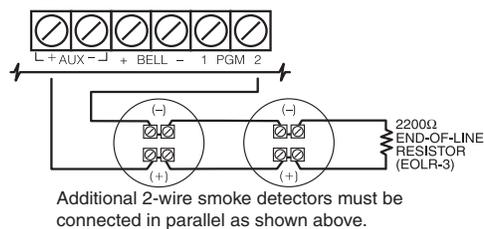
**NOTE:** The maximum number of smoke detectors on a 2-wire loop is 18. For more information on Fire zones, see section [001] Zone Type on page 27.
