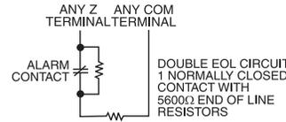
**NOTE:** If the DEOL supervision option is enabled, all hardwired zones must be wired for DEOL resistors, except for Fire and 24 Hour Supervisory zones. Do not use DEOL resistors for Fire zones or 24 Hour Supervisory zones.
