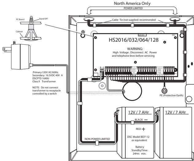
**NOTE:** Wire entry for power limited wiring must be separated by a different entry access from non-power limited wiring.
