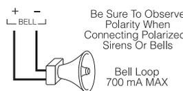
The Bell output is supervised and power limited by 2A PTC. If unused, connect a 1000Ω resistor across Bell+ and Bell- to prevent the panel from displaying a trouble. See [\*][2] on page 17.
