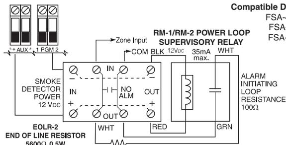
Smoke Detector must be latching type (e.g., DSC FSA 410B Series)
