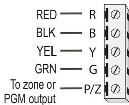
**NOTE:** When using end of line supervision, connect the zone according to one of the configurations outlined in Section 2.4.8.. End of line resistors must be placed on the device end of the loop, not at the keypad.
