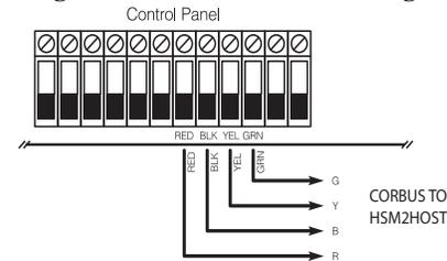
After you have completed the wiring, reconnect power to the security system. Board current draw: 35mA
