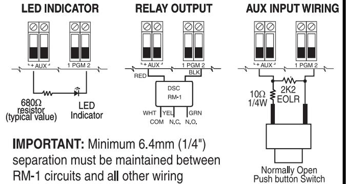
**IMPORTANT:** Minimum 6.4mm (1/4") separation must be maintained between RM-1 circuits and all other wiring
