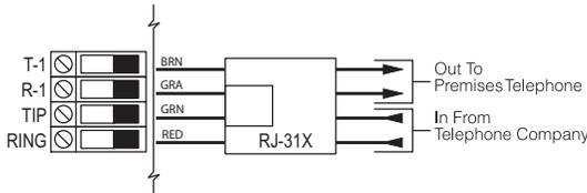
**NOTE:** Ensure that all plugs and jacks meet the dimension, tolerance and metallic plating requirements of 47 C.F.R. Part 68, Sub-Part F. For proper operation, no other telephone equipment must be connected between the control panel and the telephone company facilities.
